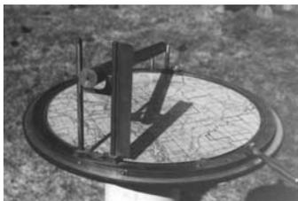
In 1915, Osborne again modified his firefinders sighting mechanism. The 1915 model featured a 0-power scope similar to those used on a rifle, instead of the original fore and aft upright sights, to peer through. Precision calibration permitted obtaining azimuth readings to the nearest minute or 1/60<sup>th</sup> of a degree; and a vertical angle reading to 1/10<sup>th</sup> of a degree. Leupold-Volpel & Co. produced several hundred of the 1915 Osborne Firefinders.
